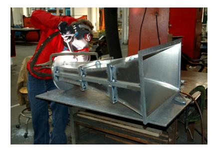
The aluminum skin of the 80 Hz midbass horn is reinforced by 56 machined aluminum ribs for stiffness and resonance control. It is hand-welded by skilled craftsmen and takes 4 month to complete.
